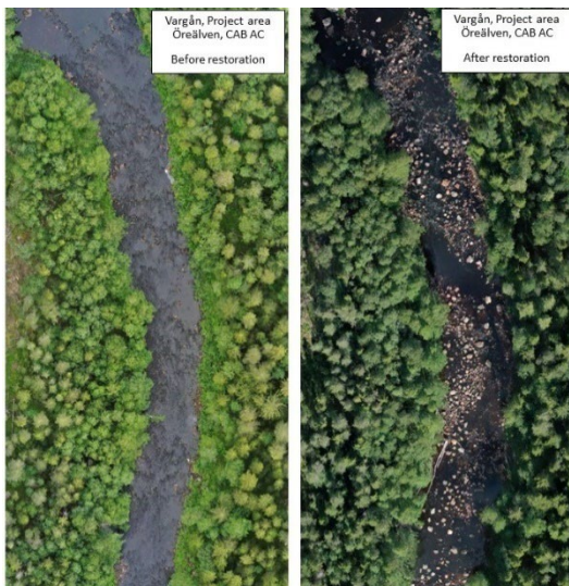
Figure 23. Example of drone documentation, before and after restoration. When calculating rewetted area, the area of the river is assessed with GIS, and new area is subtracted by the old area to get the increase.
