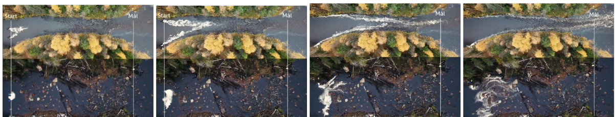
Figure 24. D1.1 Hydrology, (still images cut from film) from above. Sawdust released before (above) and after restoration (below). Still images captured at 10 seconds, 20 seconds, 30 seconds and 40seconds.
